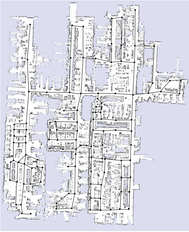
Fig. 3. Grid map and roadmap for the KUKA production site in Augsburg with a size of 300 \times 200 meters.
